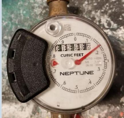
The Town's water meters are read in cubic feet, to calculate the gallons of water delivered to the home take the cubic feet reading from the water meter (first four numbers from left to right) add two zeros and multiply by 7.48. Using the reading on the meter above of 126,300  $\times$  7.48 = 944,724 gallons for the life of the meter.
