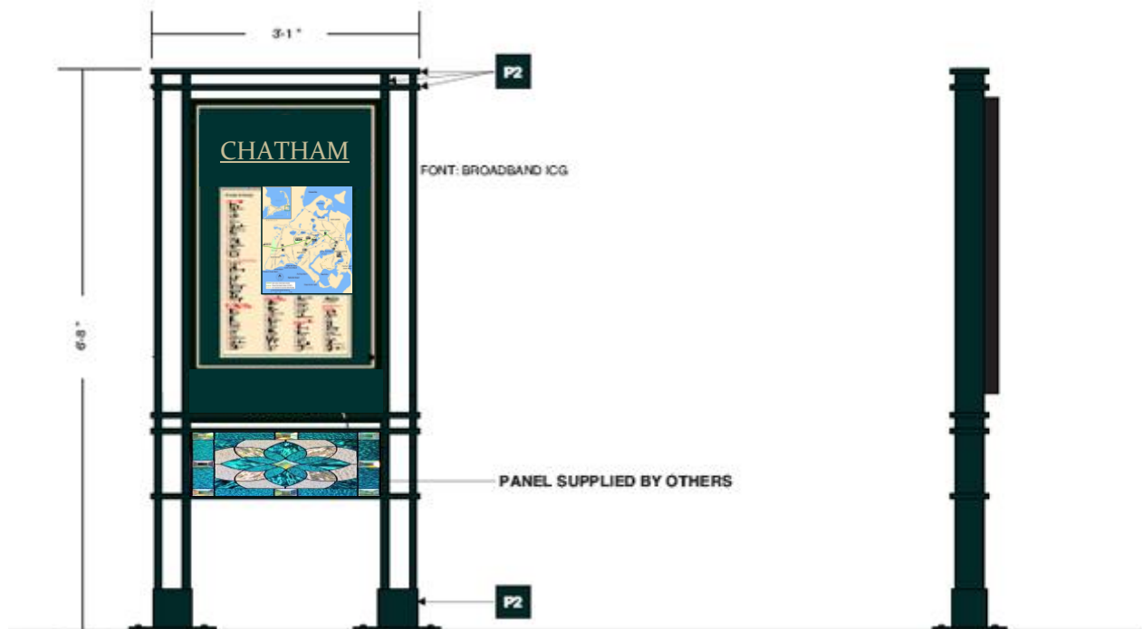
Example of wayfinding kiosk with 2 information panels
