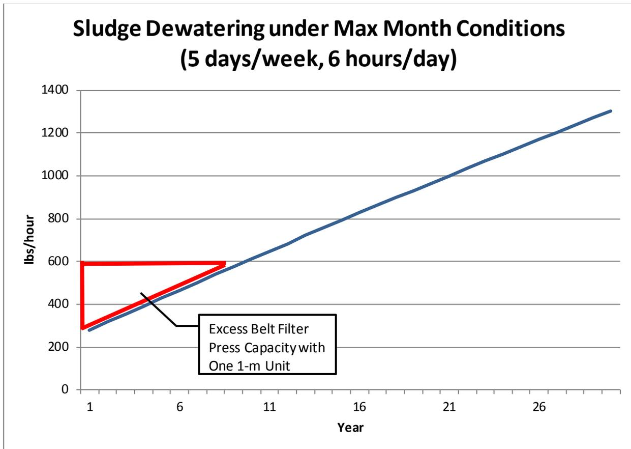
Figure 5-2 Belt Filter Press Capacities Under Maximum Month Conditions
