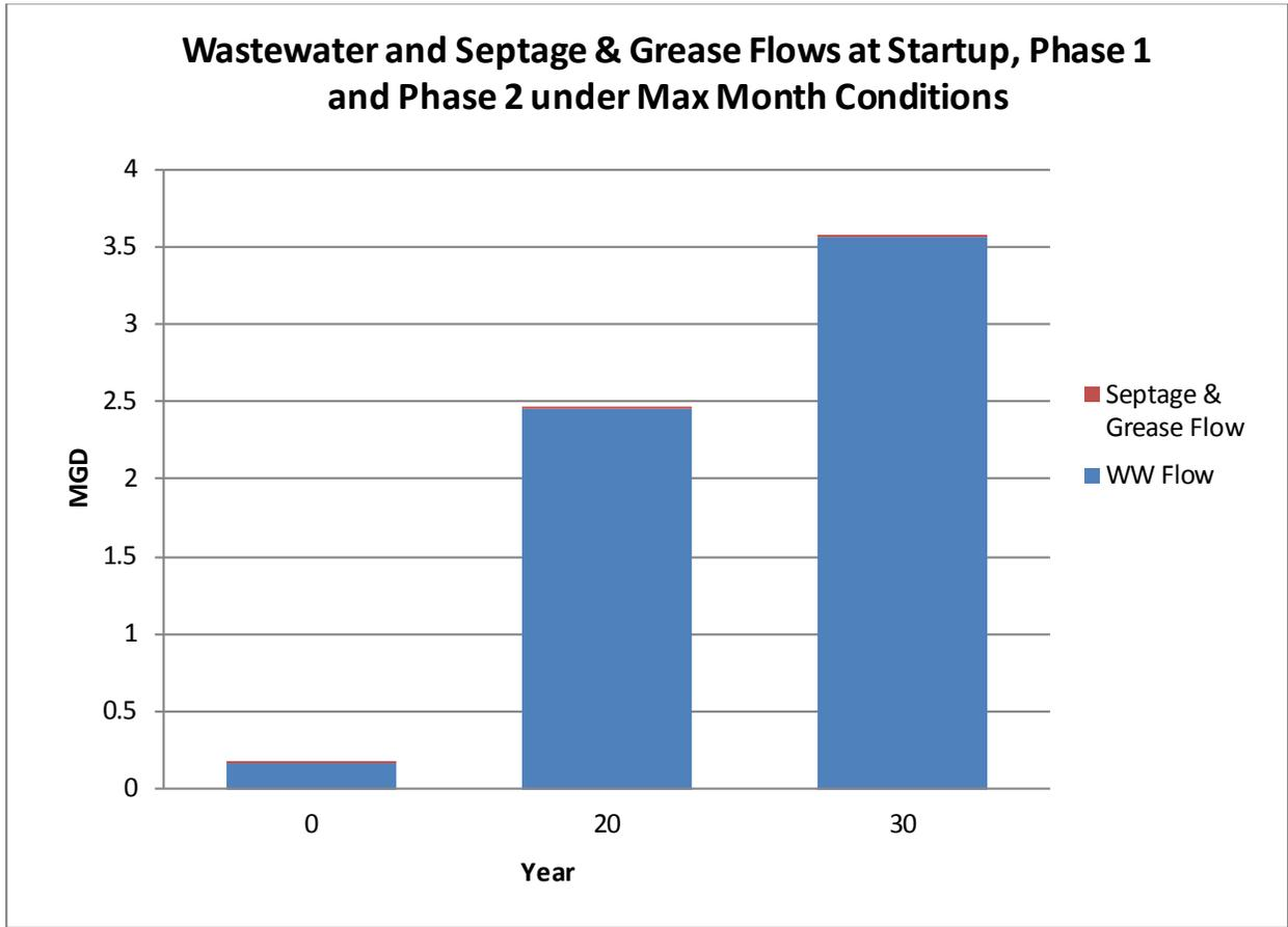
**Figure 4-1 Septage and Grease Quantities Relative to Wastewater Flows**
