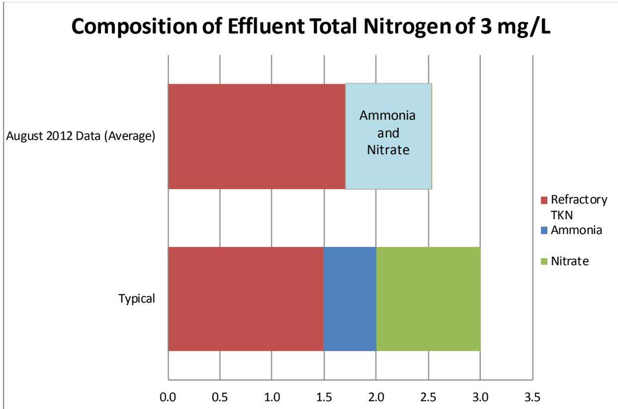
**Figure 5-4 Composition of Effluent Total Nitrogen of 3 mg/L vs. August 2012 Plant Data**
