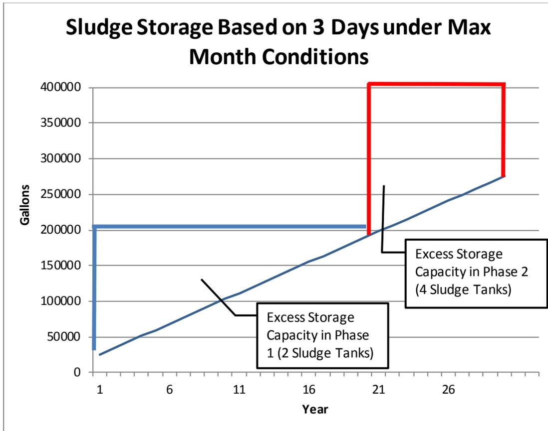
Figure 5-1 Sludge Storage Based on Three Days Under Maximum Month Conditions
