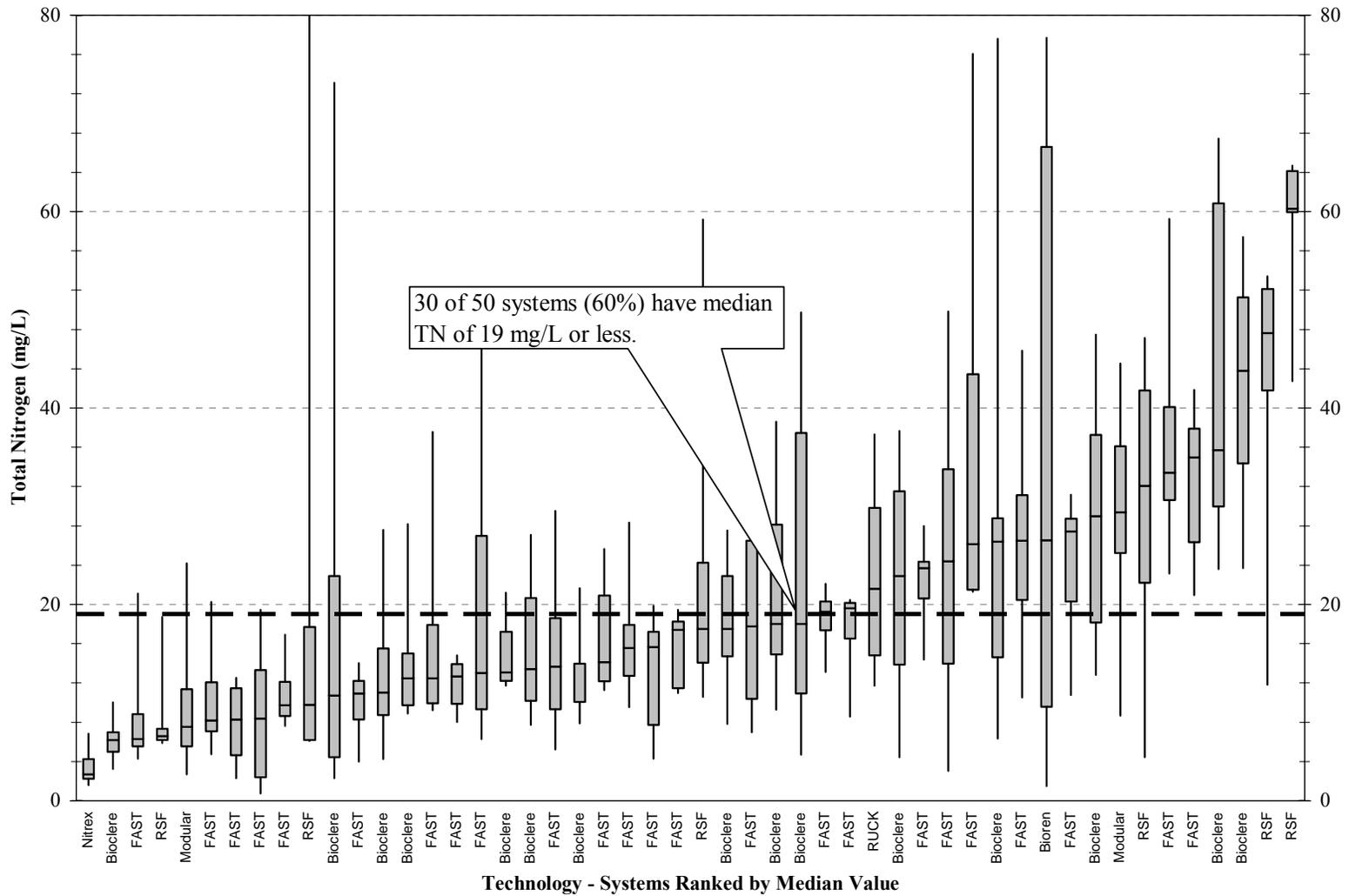
**Figure 10. Ranked median total nitrogen concentrations from multi-family I/A systems plotted with range values (only systems with  $\geq 4$  samples included). Modular= Modular FAST, RSF= Recirculating Sand Filter.**
