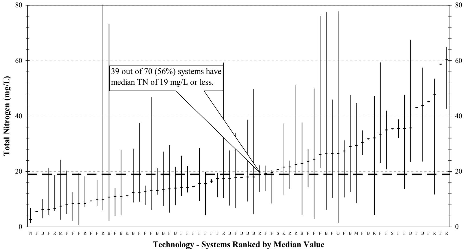
**Figure 9. Ranked median total nitrogen concentrations from multi-family I/A system technologies plotted with range values (all systems with any number of samples included). B=Bioclere®, F= FAST®, R= Recirculating Sand Filter, K=RUCK®, N=Nitrex®, S= Singular®, M= Modular FAST, O= Bioren. Systems with single sample only represented by median bar at that single value.**
