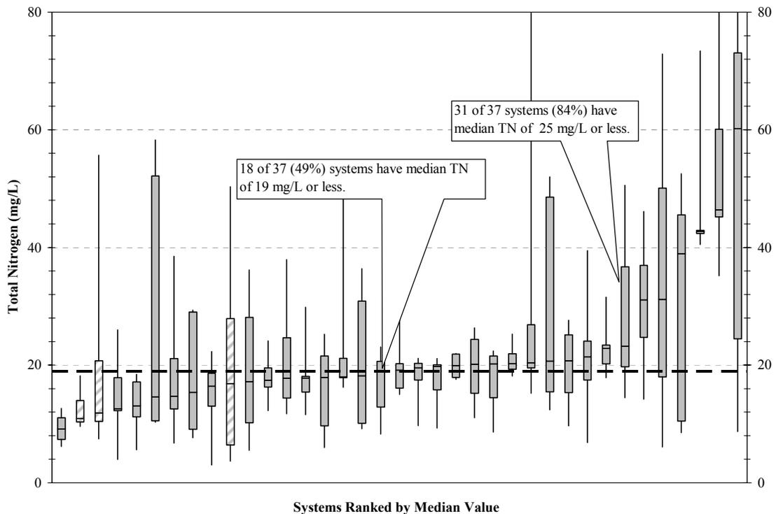
**Figure 16. Ranked median total nitrogen concentrations from single-family RSF systems plotted with range values (only systems with  $\geq 4$  samples included). Hatched boxes correspond to systems not designed by OMNI Environmental.**
