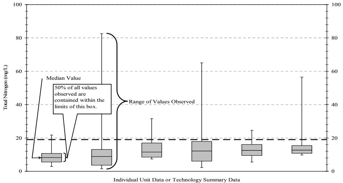
**Figure 3. Sample Box-and-whisker plot for showing central tendency of data from individual treatment units or summaries of technologies.**
