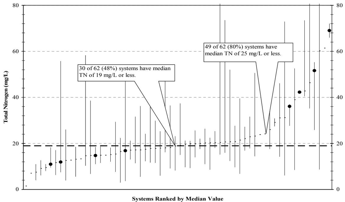
**Figure 15. Ranked median total nitrogen concentrations from single-family recirculating sand filters plotted with range values. All systems with any number of samples included. Darkened medians (●) correspond to systems not designed by OMNI Environmental.**
