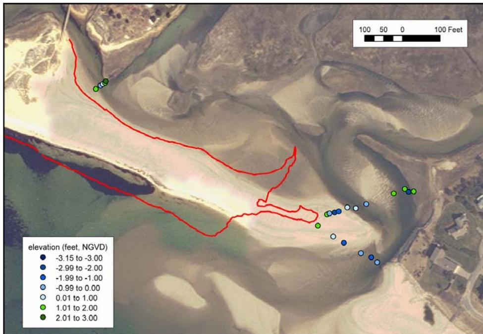
Figure 1. Plot of channel cross sections surveyed May 31, 2007 at the inlet to Bucks Creek. Survey Points and the measured GPS shoreline (solid red line) from the same day are plotted over an April 2005 Mass GIS aerial orthophoto.
