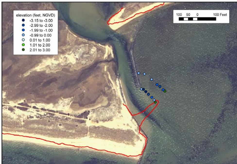
Figure 2. Plot of channel cross sections surveyed May 31, 2007 at the inlet to Mill Creek and Taylors Pond. Survey Points and the measured GPS shoreline (solid red line) from the same day are plotted over an April 2005 Mass GIS aerial orthophoto.
