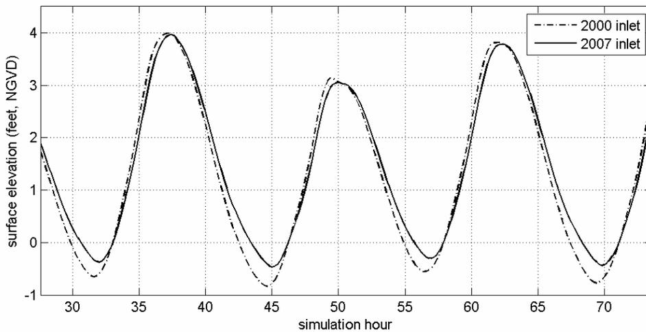
Figure 4. Comparison of modeled tides in Mill Creek, for 2000 (dot-dashed line) and 2007(solid line) inlet configurations.
