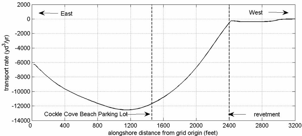
Figure 14. Net sand transport rates (cubic yard / year) along Cockle Cove Beach computed using the GENESIS model of the shoreline, for the 2005 to 2007 simulation period. Negative rates denote net sand movement to the east. Dashed lines indicate positions of features shown in Figure 11.
