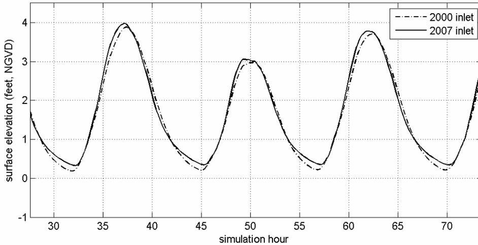
Figure 3. Comparison of modeled tides in Bucks Creek, for 2000 (dot-dashed line) and 2007(solid line) inlet configurations.
