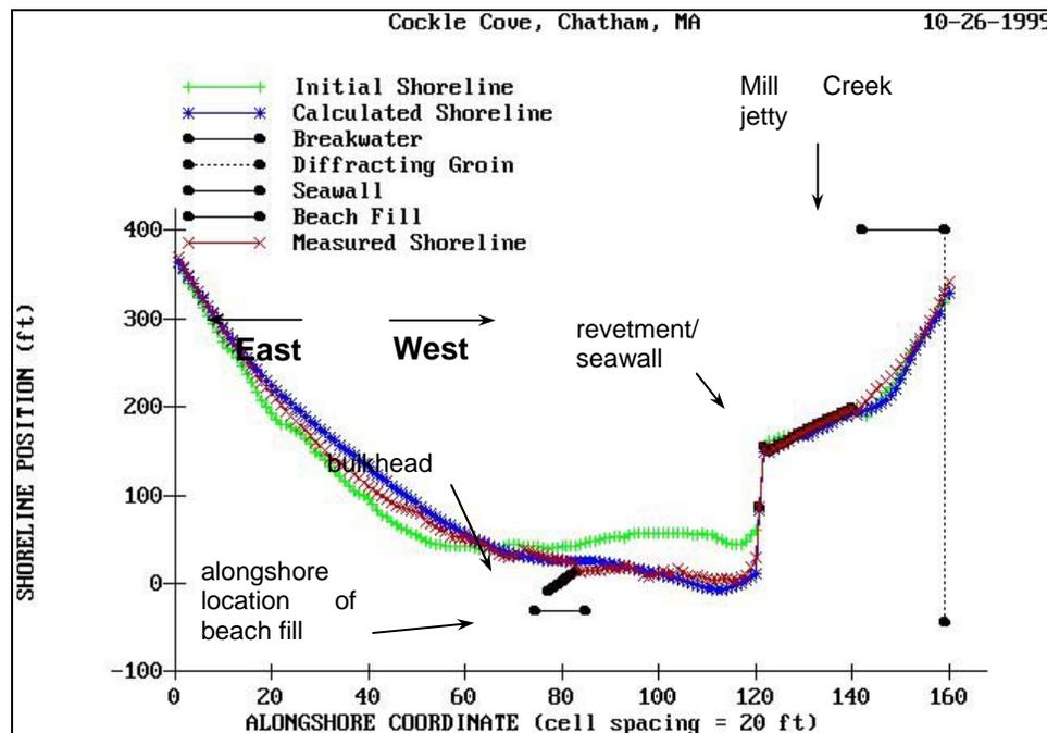
Figure 11. SMS display of GENESIS output from the original analysis of Cackle Cove Beach. Shown in the plot are model representations of structures located on the beach, as well as modeled location of recommended beach fill design. The offshore direction (south) is up in this plot.
