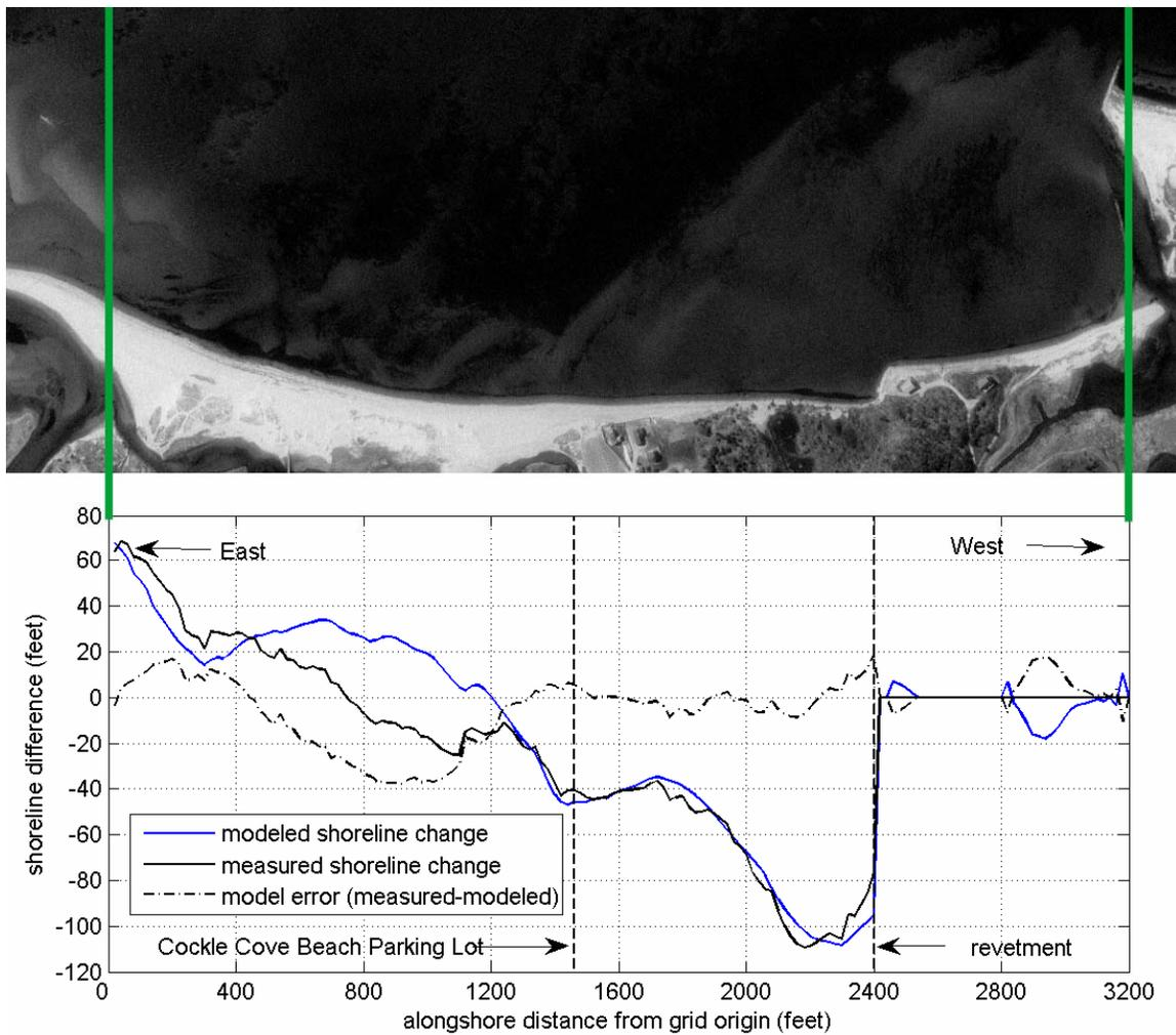
Figure 13. Aerial photo of Cockle Cove Beach shown with a plot of shoreline change from 2005 to 2007, for both measured and modeled shorelines. Difference between measured and modeled 2007 shoreline is also plotted. Solid green lines indicate the GENESIS model limits, and dashed lines indicate positions of features along the beach relative to the model grid origin.
